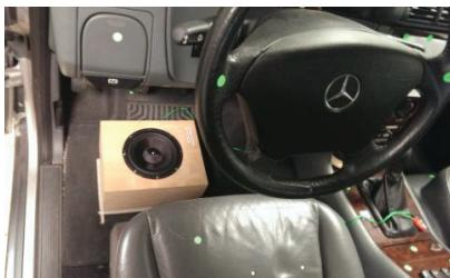
Figure 1. Loudspeaker positioning in the vehicle interior.
