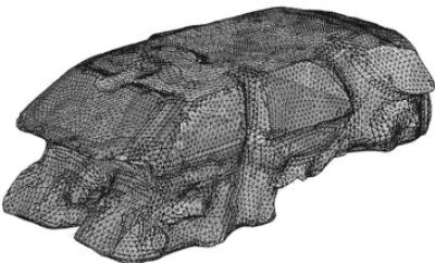
Figure 4. Surface mesh of the car cabin.
